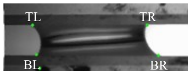
Fig. 1 Snapshot of liquid meniscus bridge between glass plates under shear, dotted edge with “TL” means position of a detected contact line at the Top – Left
