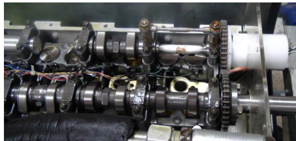
Fig 1. Instrumented engine for camshaft friction and tappet rotation measurement.
