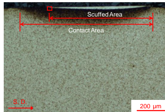
Fig. 1 Optical micrograph showing the overview of the subsurface material during scuffing. Etching condition: 2 vol.% nital, 25 seconds.
